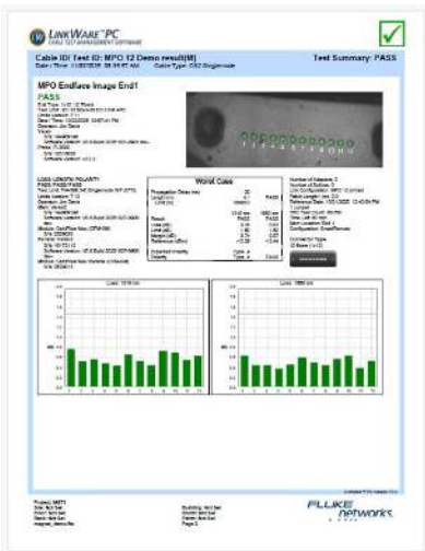
LinkWare PC report showing end face image and loss results (including PASS for each) for a 12-fiber MPO cable.
