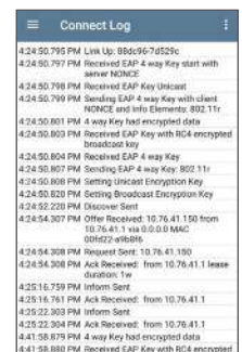
Connect Log shows roam/association process
