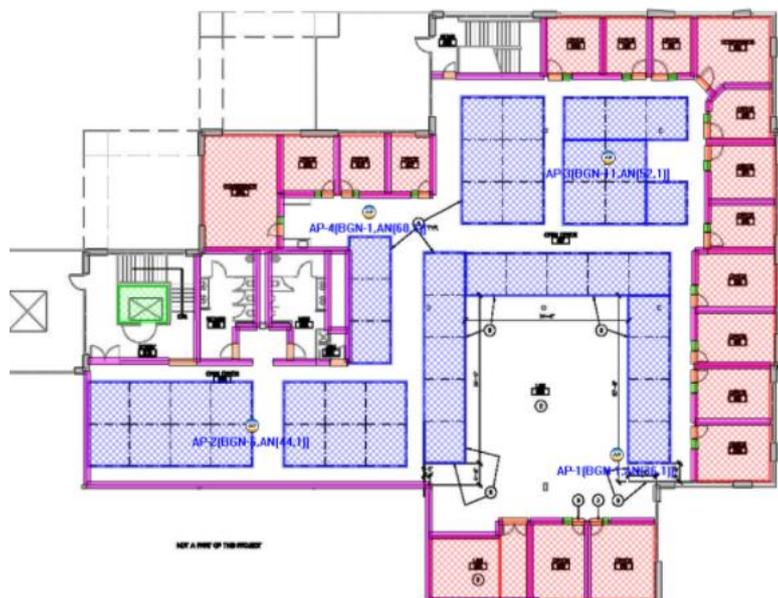
This example shows how a floor plan is marked out with the wall types and also the places where the customer does (blue hashed) and does not (red hashed) want the APs to be located.
