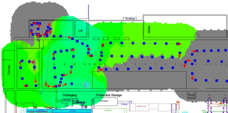
This survey data to the left shows the coverage of a single AP in a factory.
