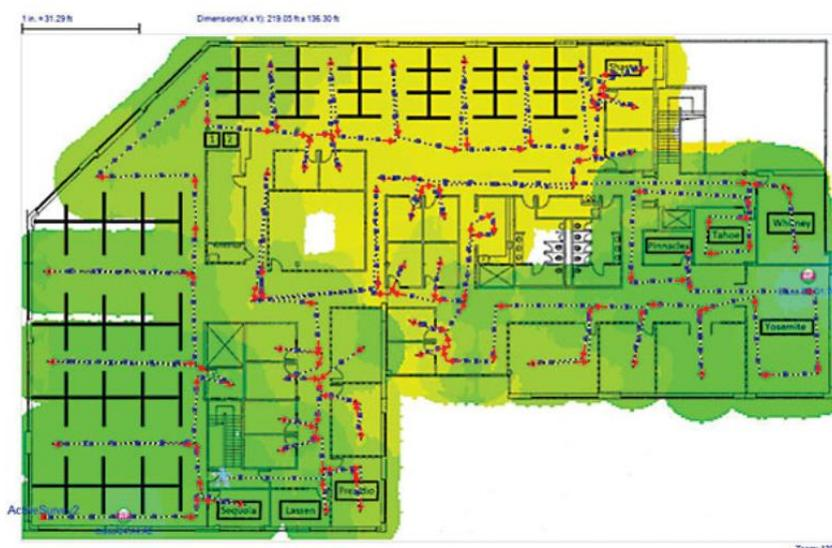
The survey image to the left here shows where you have walked (the dotted lines), whilst the differing colour shading indicates the signal strength.
