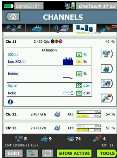
Figure 14. Visibility into each Wi-Fi channel, showing bandwidth occupied by 802.11 and non-802.11 traffic
