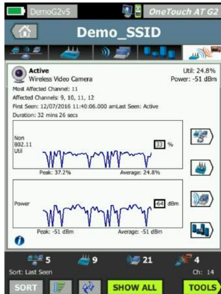
Figure 16. Detailed information about a specific interference source
