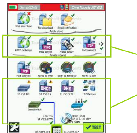
Figure 1. The AutoTest provides a comprehensive measurement of network performance from the end user point-of-view, from cable, to services and applications (Test result from OneTouch AT with G2 Modules for both Wired and Wi-Fi network shown)
