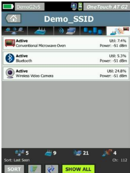
Figure 15. Unique Interferer analysis classifies sources of non-802.11
